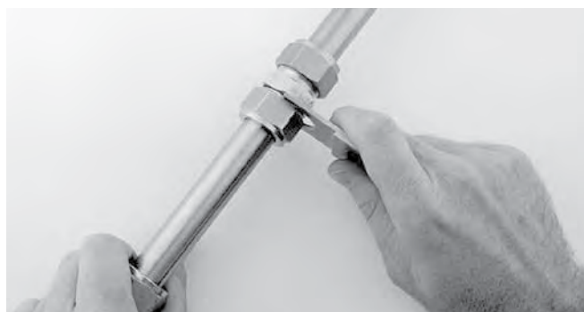
When fitting is properly tightened, gap gage should not fit between nut and shoulder of body.
